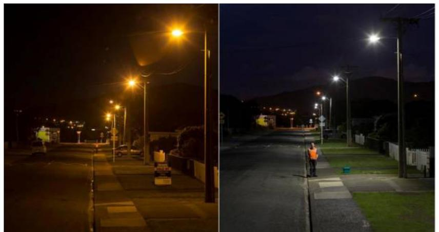
How Findlay St, Tawa looked before and after its conversion to LED street lighting in 2014 – courtesy of Stuff.
